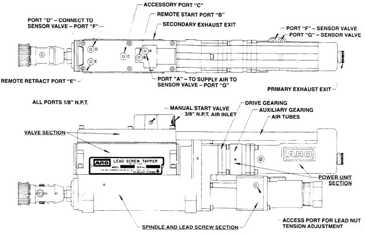
The three basic sections of the Lead Screw Tapper are arranged for efficient maintenance. The following is a brief description of the sections and their functions.
